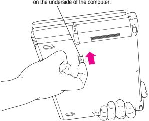
To unlock the module, slide the latch on the underside of the computer. 4 Hold the module by the gripping surface and pull it out of the computer.
